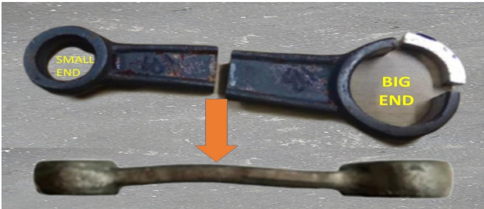
Figure 5 Placement for the metallography analysis
