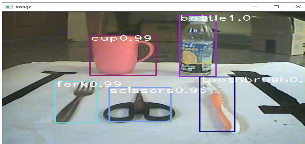
Figure 11: Sample of YOLOv8n Detection Results
