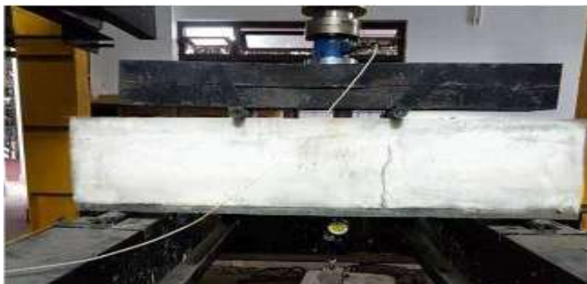
Figure 3: (Retrofitted beams with SIFCON laminates) illustrates how SIFCON has been applied to structural members for improved performance
