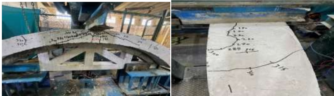
Figure 10: Failure of control beam (CTA.T 0 P 0 P 0 )
