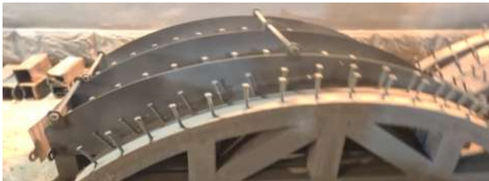
Figure 9: (Shear connector distribution) highlights the role of shear connectors in stress transfer
