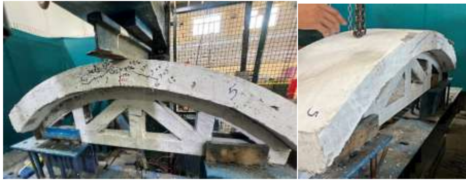
Figure 12: Failure of SIFCON-enhanced beam (CTA.T 3 P top P 10 )
