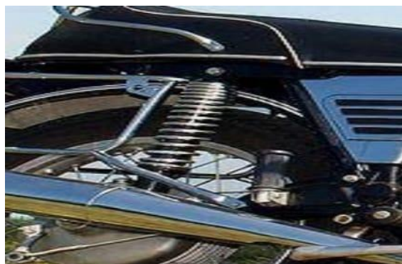
Figure: 1 Rear shock absorber and spring of a motorcycle
