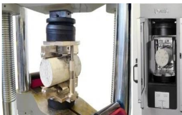
Figure 2: Split Tensile Strength Testing
