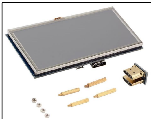
Figure 3: 5-Inch LED Display Used for Feedback
