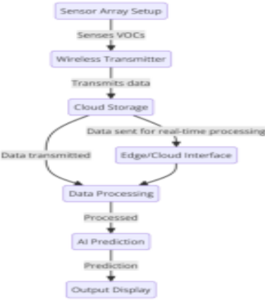
Figure 2: Data Flow in an IoT-Enabled E-Nose System
