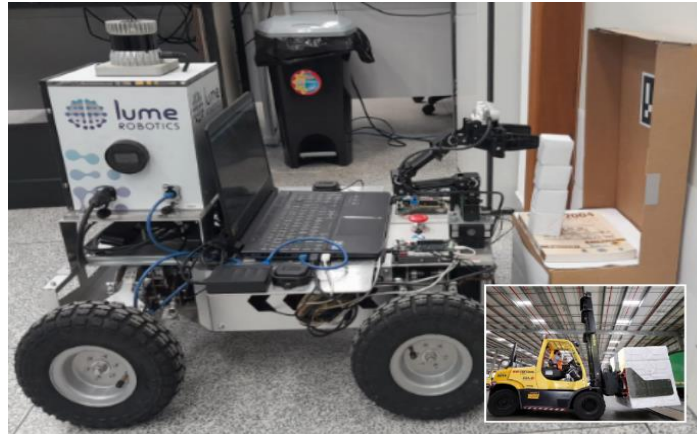
Figure 2: Illustration of the designed robot Hercules and the real forklift it aims to emulate.
