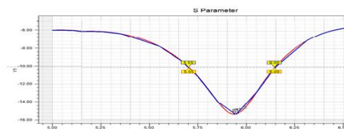
Fig. 12. S11Return Loss for Antenna Measured and simulated
