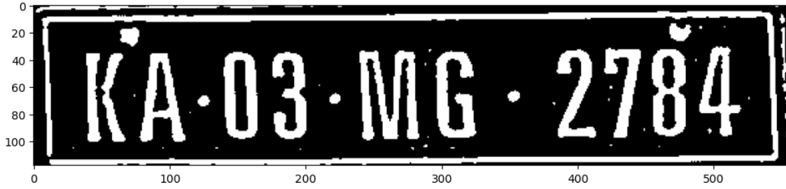
Fig. 7: Input image after Adaptive thresholding
