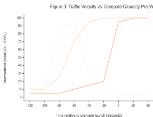
Figure 3: Time-series graph demonstrating the derivative of login velocity peaking 60 to 90 seconds before backend manifest demand, triggering the burst pre-warming sequence that absorbs the load.
