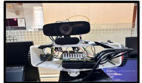
Figure 10: Pi camera with Arduino setup
