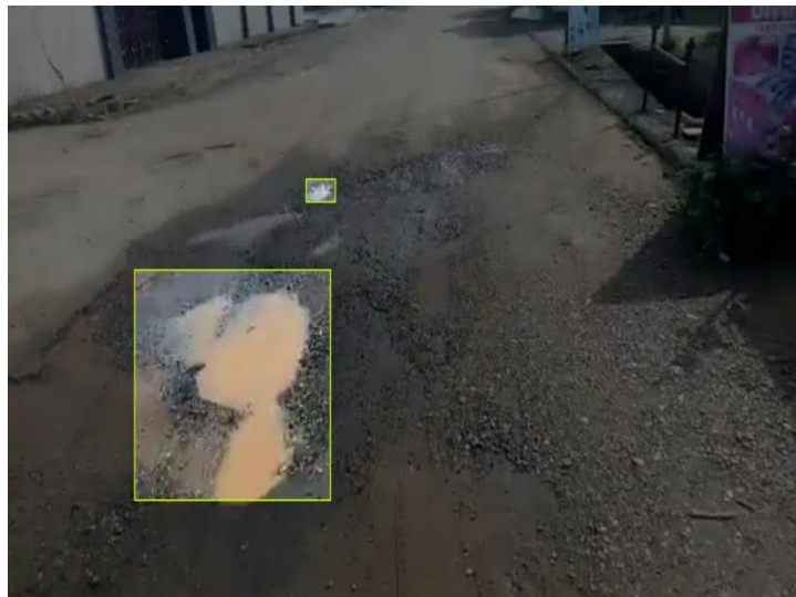
Figure 1: YOLOv8 Pothole/Crack Detection Example
