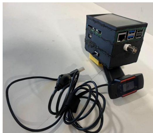
Fig 6. 3D-Printed Prototype Enclosure with Camera, TFT Screen, and Other Components (Side View)
