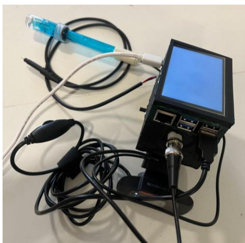
Fig 7. 3D-Printed Prototype Enclosure with Camera, TFT Screen, pH Sensor, and TDS Sensor
