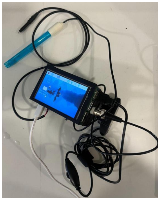
Fig 12. Portable Water Quality Monitoring System
