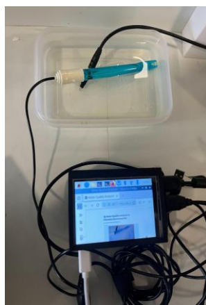
Fig 13. Portable Water Quality Monitoring System with its TDS and pH Sensors Dipped in Water with Little Oil
