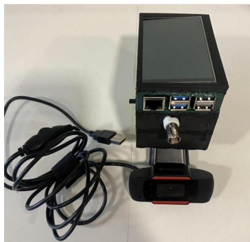
Fig 5. 3D-Printed Prototype Enclosure with Camera, TFT Screen, and Other Components (Front View)
