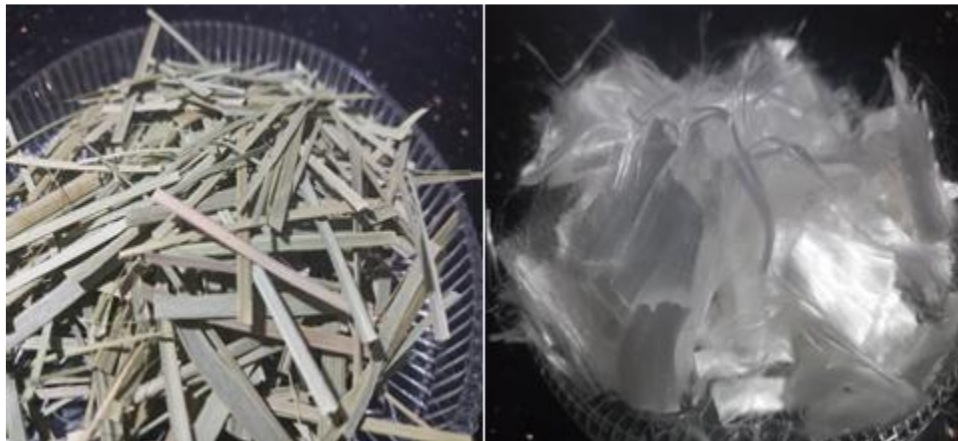
Figure 1. Types of Fibres used; (a) Doum Fibres (DF), (b) Polypropylene Fibres (PPF)
