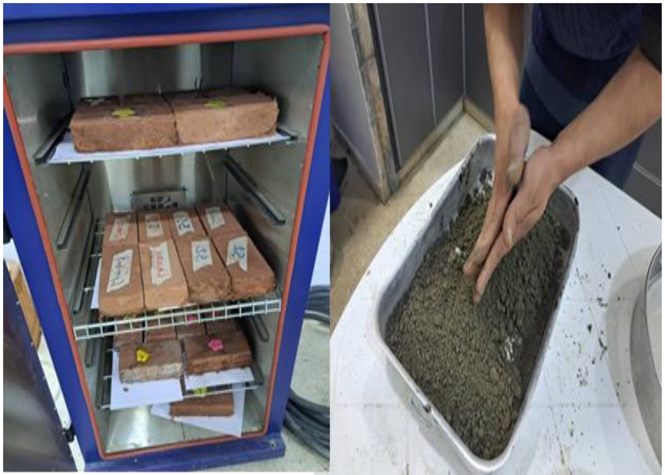
Figure 2. Block Fabrication and Curing
