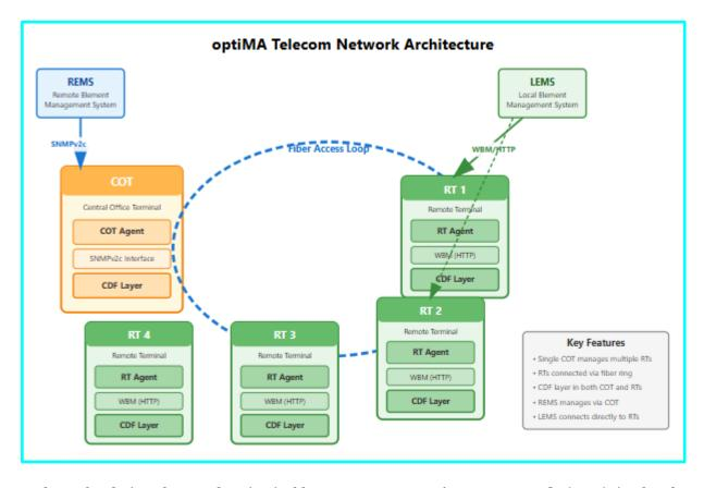
To keep the design clean and maintainable, a **Common Device Framework (CDF)** is placed underneath both the SNMP and WBM agents in the COT and RT. Here's how it works in practice:
