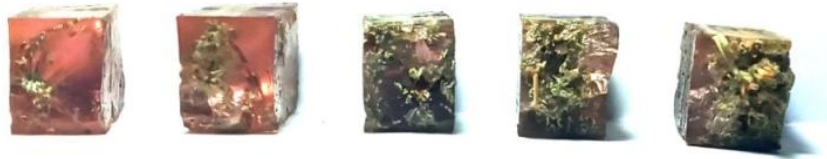
Figure 11: Cross Sections of Charpy-Impacted Specimens.
