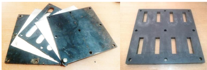
Figure 3. Mold of tensile specimens (left) and median piece of mold for impact test specimens (right)
