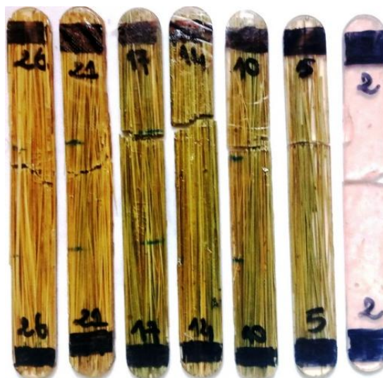
Figure 5. Samples of tensile test specimens with different weight percentage of Diss fiber after being tested
