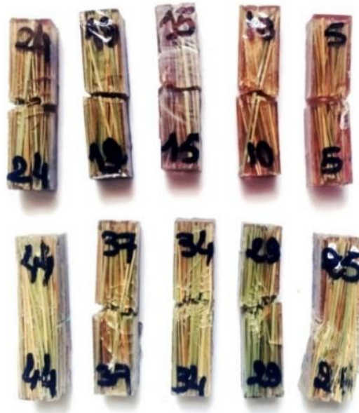
Figure 9. Samples of impact test specimens with different weight percentages of Diss fiber after being tested
