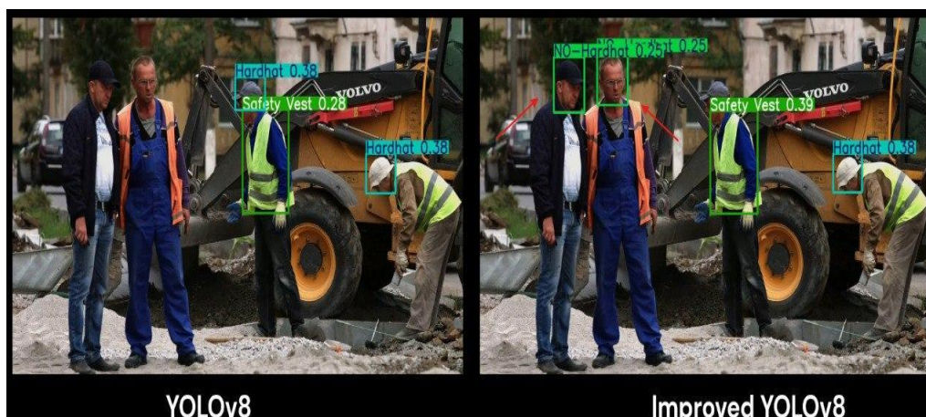
Figure 7: Safety Gear Detection: Comparison Between YOLOv8 and Improved YOLOv8.
