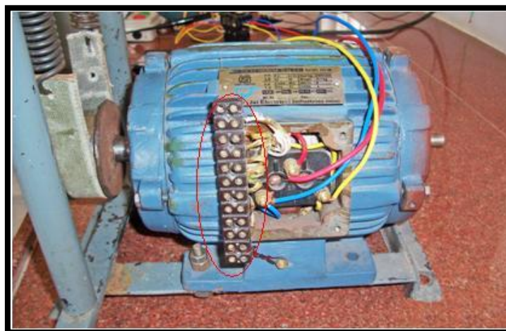
Figure 4: Tapping arrangement on Induction Motor
