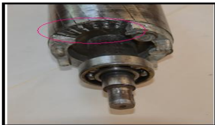
Figure 5: Induction motor with broken rotor bars
