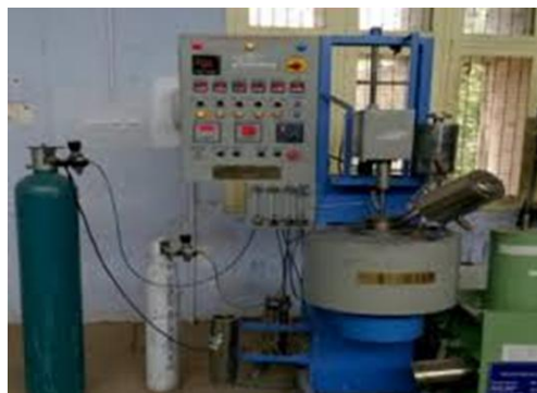
Figure 1 Stir-casting set-up used to produce Al6063/SiC/B 4 C/FA hybrid composites
