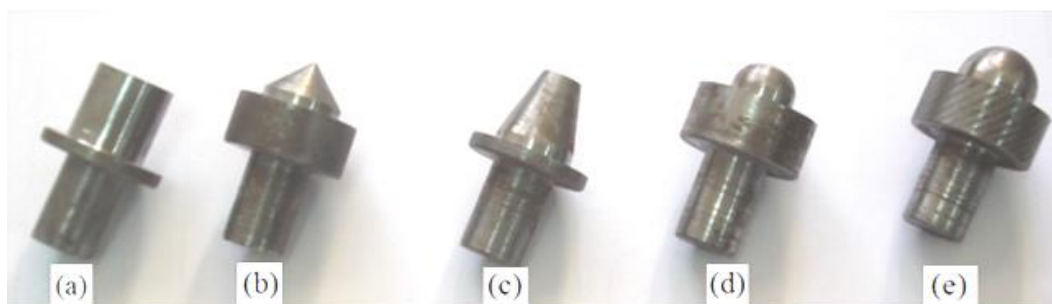
Figure 4: The different indenters' geometry used in this study: (a) Cylindrical, (b) Conical, (c) Truncated cone, (d) Hemispherical 16mm and (e) Hemispherical 20mm.
