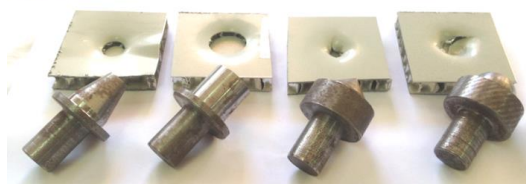
Figure 8: Failure modes of indentation test for each indenter.
