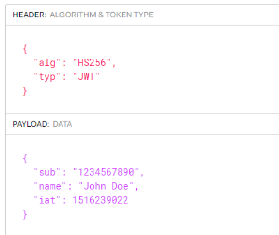
Figure. 4 The header, payload of JWT
