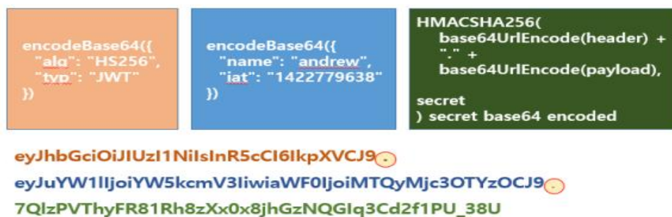
Figure. 3 The structure of JWT
