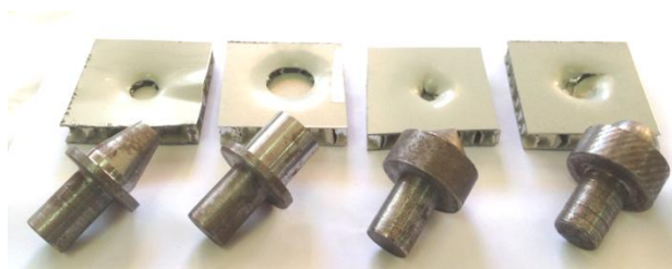
Figure 8: Failure modes of indentation test for each indenter.
