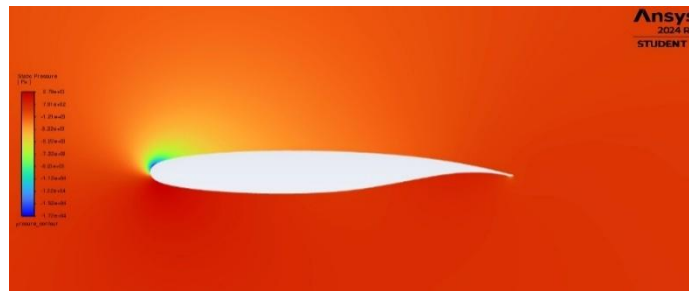
Figure 10. Pressure Contour of NACA SC (2)-0714 at 11° angle of attack
