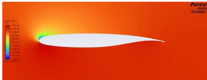
Figure 14. Pressure Contour of NACA SC (2)-0714 at 17° angle of attack
