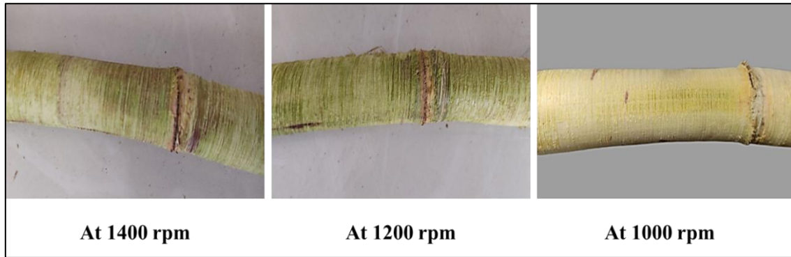
Fig. 3: Peeled cane at operation of 1400, 1200 and 1000 motor rpm
