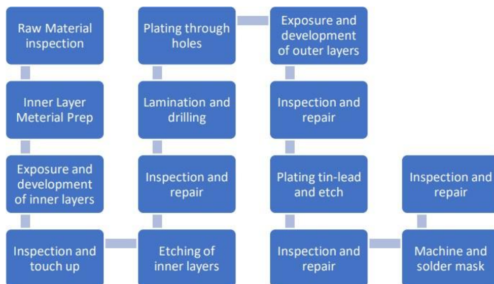
Fig.1.1: Printed Circuit Board Manufacturing Flow Diagram
