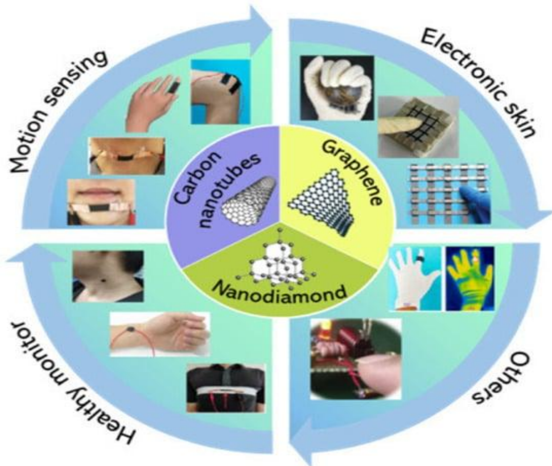
Fig 10. Application of strain sensors based on carbon nanotubes, graphene, and nanodiamond in harsh environments.
