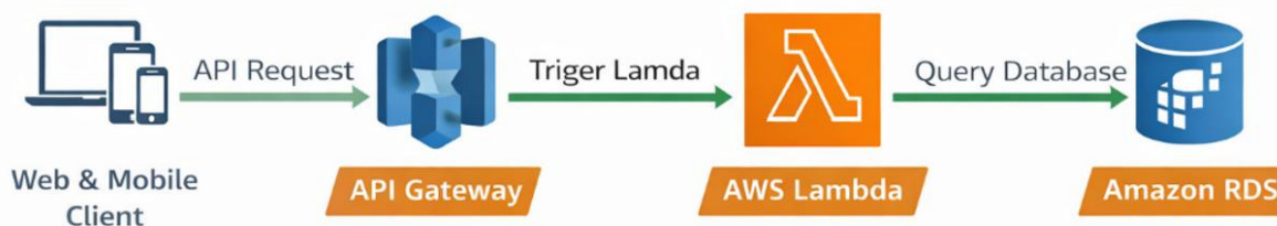
Figure 2: Request flow diagram illustrating client interaction through API Gateway to AWS Lambda and Amazon RDS.
