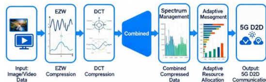
Fig. 6 : Data Flow Diagram for the Integrated EZW-DCT Compression and Dynamic Spectrum Management Framework in 5G D2D Communication
