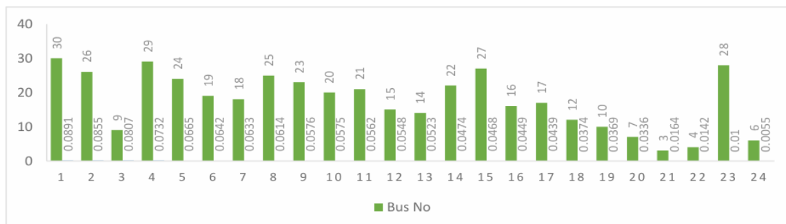
Figure 3 L-index values for the IEEE 30-bus system.
