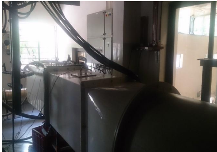
Fig 7 cooler testing in wind tunnel
