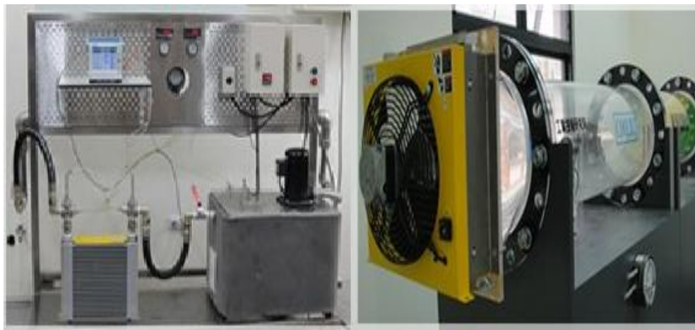
Fig.8 Cooler leak and performances testing
